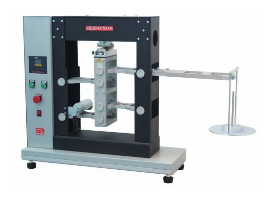
USED TO DETERMINE STRENGTH OF PROTECTIVE CLOTHING AGAINST CUTTING
